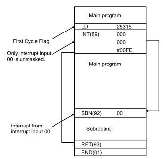
**Note** Depending on the setting of DM 6621 in the PC Setup, Host Link servicing, Remote I/O servicing, Special I/O Unit servicing, and individual instruction execution will be completed before the subroutine is executed. Refer to page 255 for details.
